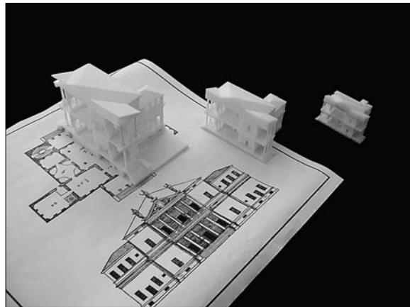
FIGURE 14-4 Physical Model produced by a 3-D printer.
